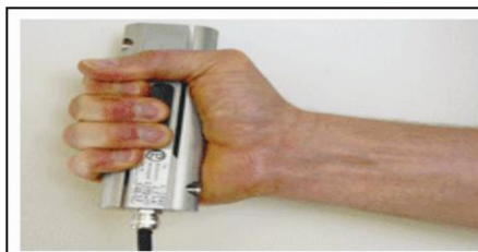
Fig. 2a: Volunteer squeezing the MLT004/ST Grip Force Transducer
